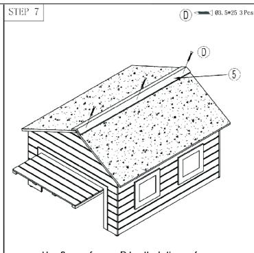
Use 3 pcs of screw D to attach the roof cap.
