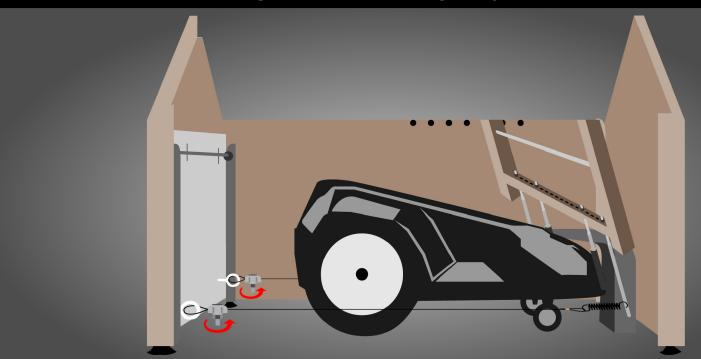
4. Test: Try to make the robot dock now, and if it is successful then the installation is done.
