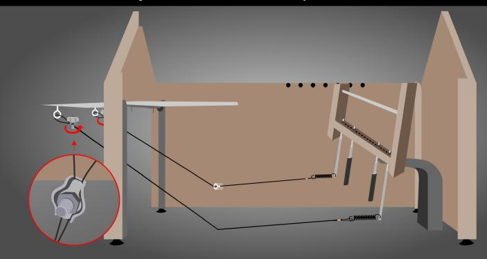
3. Open the door so it is horizontal, and use the wire to connect the mechanism to the door. The mechanism must be in a forward position towards the door, as shown in the picture. Use the adjuster to tighten the wire to the door.
