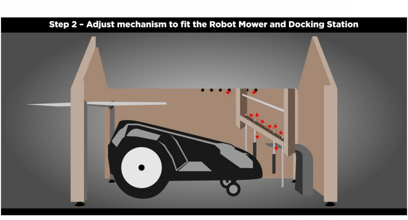
2. Fit the mechanism into the garage and adjust the 2 center poles, so it will match the robot size and docking station. At the top of the side panels you will be able to adjust the mechanism forward or backward. These adjustments will help you achieve a perfect fit for your Robot Mower.
