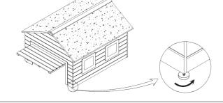
Adjust the level feet below the garage, so the port does not touch the ground/grass
